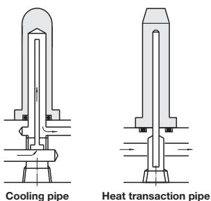
Please use cooling pipes or heat exchange pipes so as to increase cooling efficiency for the tip section of center pins.
