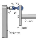
Attach and fix the thread of the suction bracket to the screw hole of
