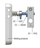
Attach and fix the cylindrical part of the suction bracket to the pipe holder (AT-PHC).
